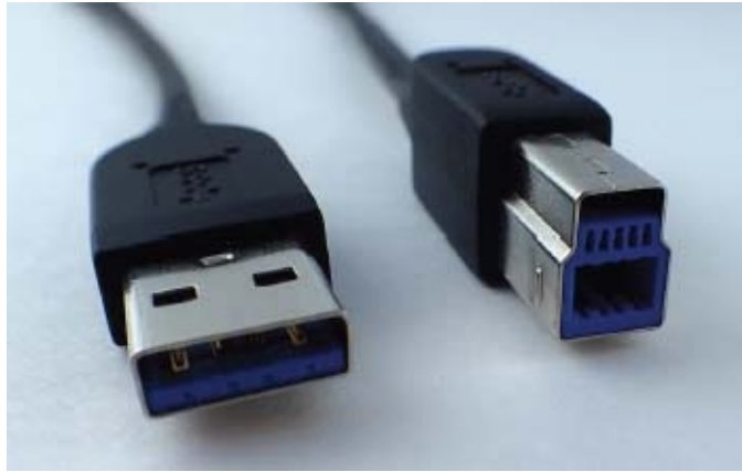
Figure 20-9. A USB 3.0/3.1 Standard-A plug (left) fits a USB 2.0 receptacle, but a USB 3.0/3.1 Standard-B plug (right) requires a USB 3.0 or USB 3.1 receptacle. The plugs shown are USB 3.0 plugs.
