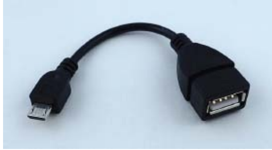
Figure 21-4. This adapter enables connecting an OTG device with a Micro-AB receptacle to a device that uses a captive cable or a detachable cable with a Standard-A plug.
