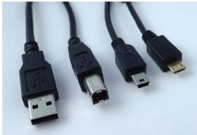
Figure 20-6. Approved cable plugs include (from left) Standard-A for hosts and Standard-B, Mini-B, and Micro-B for devices.
