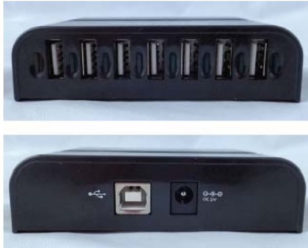
Figure 16-1. The front of this hub (top) has seven downstream-facing ports with Standard-A receptacles on the front, and the back (bottom) has an upstream-facing port with a Standard-B receptacle and a power connection.
